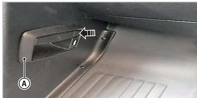
Fig.5.9 - Bonnet opening lever - Type B
