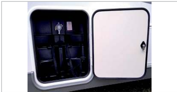
Fig.6.26 - Gas cylinder compartment
