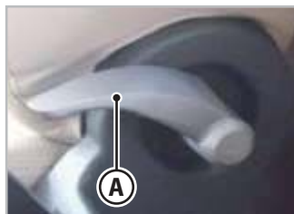
Fig.3.4 - Backrest adjustment control
