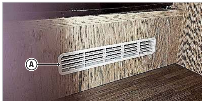
Fig.6.1 - Permanent ventilation openings
